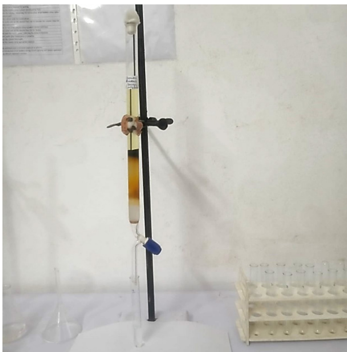
Figure 1: Isolation of components by column chromatography.
